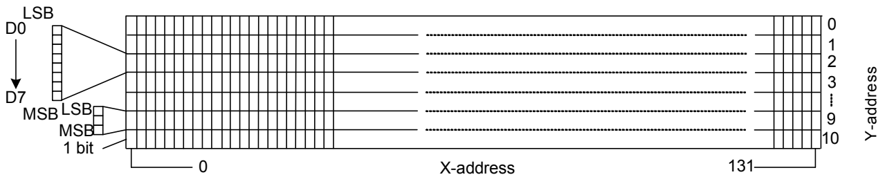
Figure 14 RAM format and addressing, if DO=0
