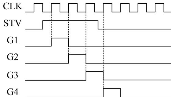
Note1: The Output Turn-On Timing will change following by Start Pulse Waveform.
