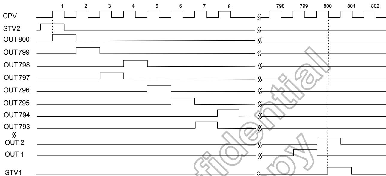
**H. Example of input/output timing (MODE1=H, MODE2=H, SEG1=H, SEG2=L,
