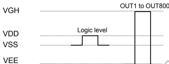
The logic levels of CPV, L/R, OE, /XAO, MODE1, MODE2, SEG1, SEG2, EVEN, STV1 and STV2 have to swing between VDD for "H" and VSS for "L".
